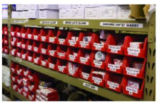
The Hardware Box (top) and bins are stocked automatically by Grunau's vendor. Hardware boxes serve all trades on a jobsite, and are an organized way to carry a minimum/maximum of miscellaneous items.
